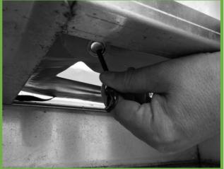
Step 7: hook the plastic hook to the upper side walls of the crate holder.
