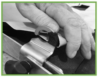
Step 6: push the plastic hook down with one hand and grab it trough the crate holder with the other hand.
